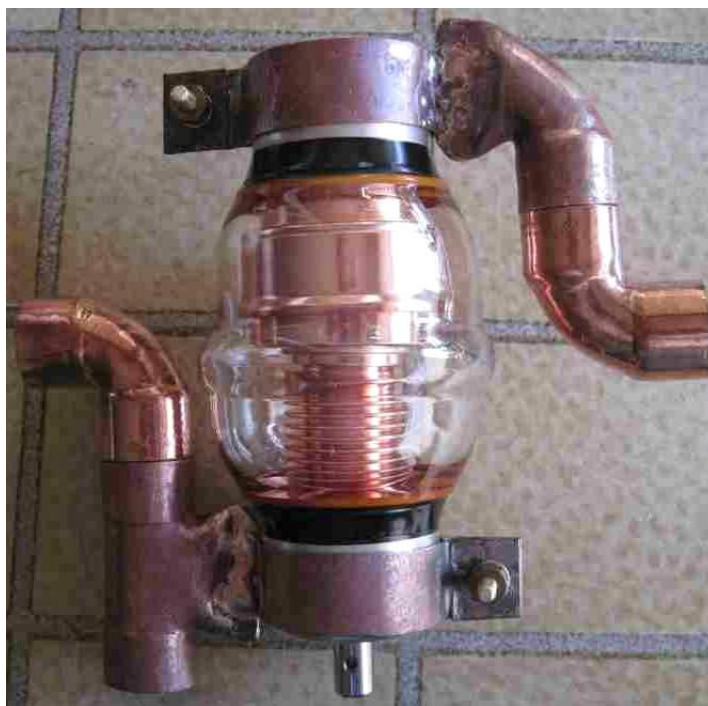
Figure 13 Homebrew capacitor clamps with silver-soldered copper fittings
