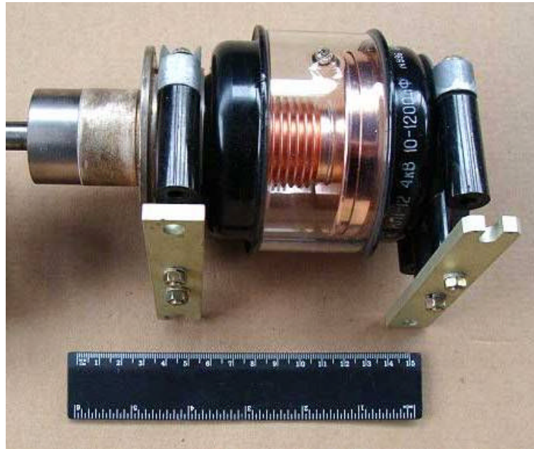
Figure 14 Russian Mil-style vacuum variable with integral clamps
