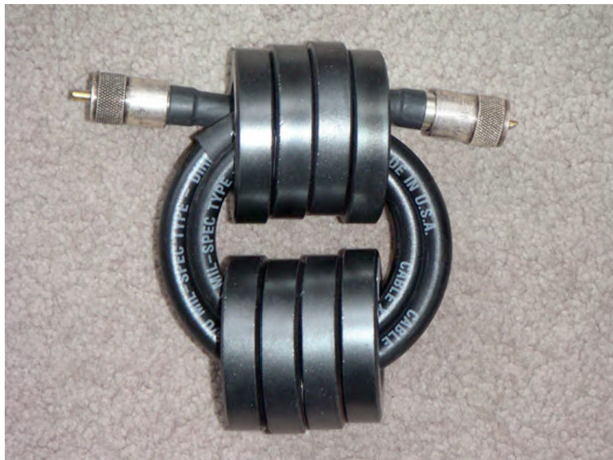
Figure 7 Multi-turn high power common-mode choke balun
