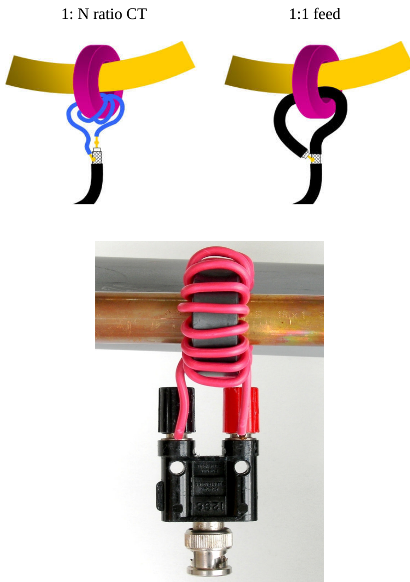
Figure 12 Conceptual and practical realisation of transformer coupling
